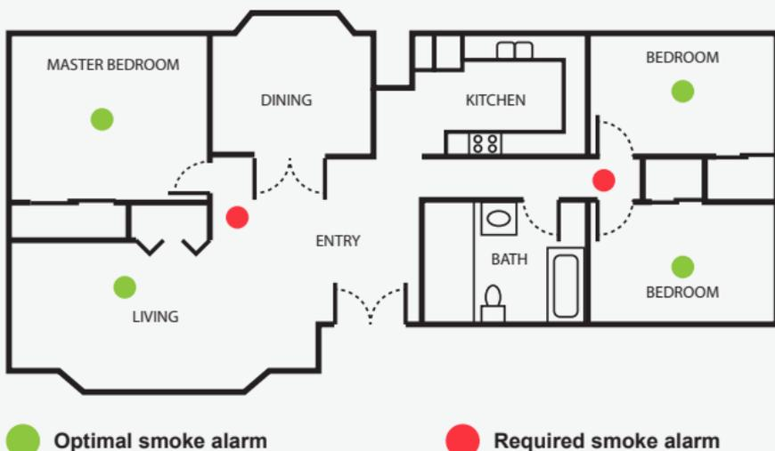
For optimum smoke detection, it is recommended that each smoke alarm is placed on the ceiling, close to the centre of the room, and at least 30cm away from the wall. Keep away from what is known as dead air space where walls and ceilings meet. Smoke alarms may not operate in these areas.
